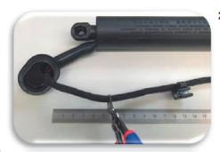
Cut the wiring harness of the original drive about 5cm (2 inches) behind the grommet.
